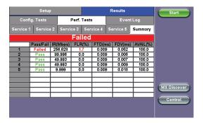
Simple summary Pass/Fail results tables and drill down capability with detailed measurements (Frame Loss, Frame Transfer Delay, Frame Delay Variation, Availability) for each service.
