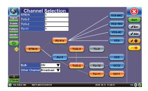
PDH/DSn client can be multiplexed and mapped into SDH/ SONET.
